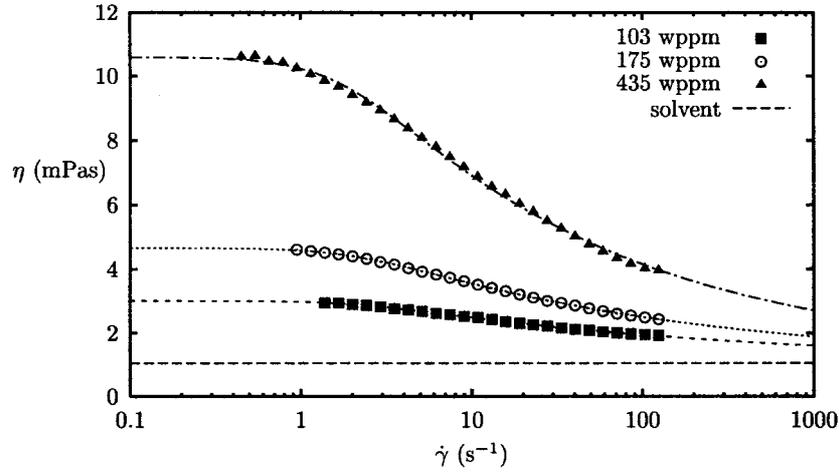
Figure 2. Viscosity as a function of shear rate for the three polymer solutions used in the LDV experiments. Symbols: measurement; lines: fit.
