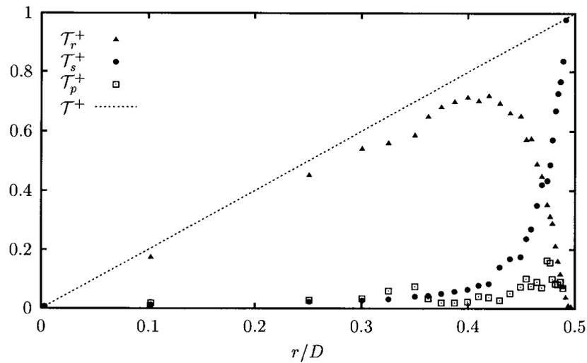
Figure 10. The various contributions to the shear stress as a function of the pipe radius for the 20 wppm solution [12].  $\mathcal{T}_r^+$ : Reynolds stress;  $\mathcal{T}_s^+$ : solvent stress;  $\mathcal{T}_p^+$ : polymer stress;  $\mathcal{T}^+$ : (theoretical) mean shear stress.  $Re_w \approx 11600$ .
