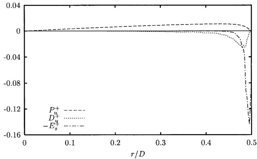
Figure 14. The various mean flow energy budget terms for water.  $Re \approx 9600$ .
