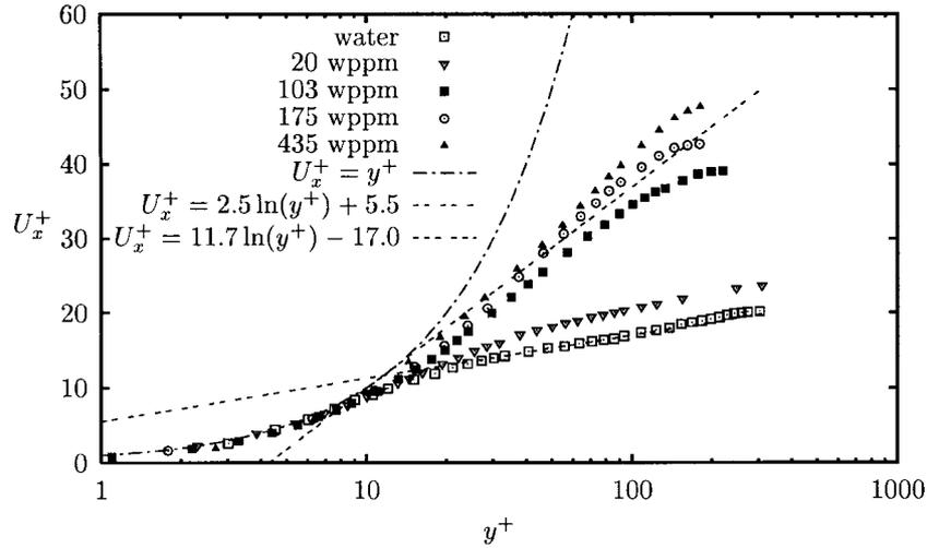
Figure 4. LDV measurements of the axial mean velocity in terms of wall units for water and for the polymer solutions. The lines are the profiles of Equations (13), (14) and (15). Flow conditions are given in Table III.
