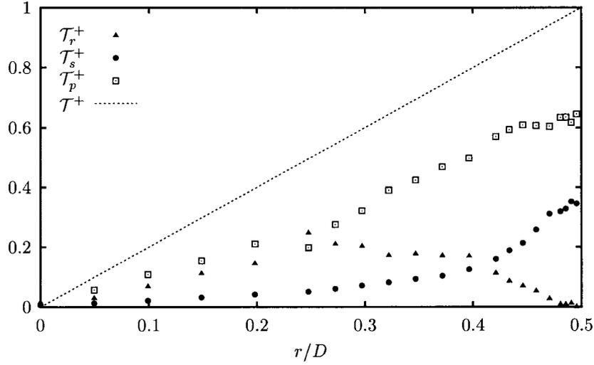
Figure 13. The various contributions to the shear stress as a function of the pipe radius for the 435 wppm solution.  $\mathcal{T}_r^+$ : Reynolds stress;  $\mathcal{T}_s^+$ : solvent stress;  $\mathcal{T}_p^+$ : polymer stress;  $\mathcal{T}^+$ : (theoretical) mean shear stress.  $Re_w \approx 10800$ .
