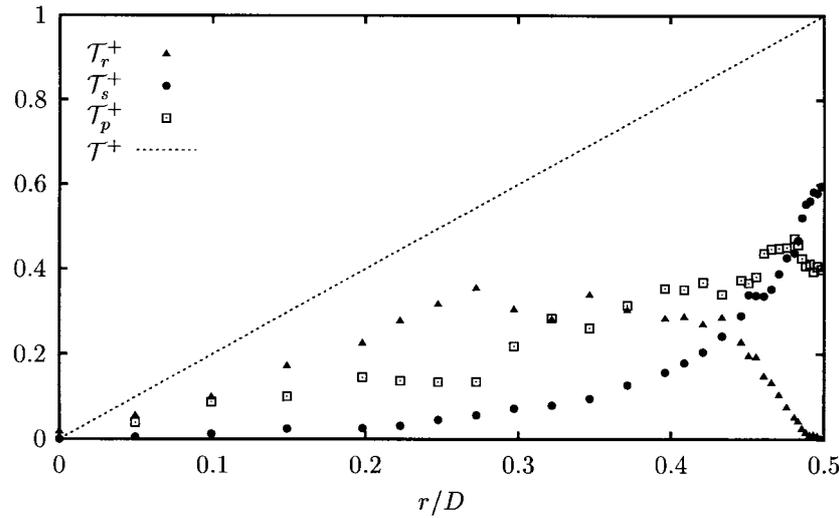
Figure 11. The various contributions to the shear stress as a function of the pipe radius for the 103 wppm solution.  $\mathcal{T}_r^+$ : Reynolds stress;  $\mathcal{T}_s^+$ : solvent stress;  $\mathcal{T}_p^+$ : polymer stress;  $\mathcal{T}^+$ : (theoretical) mean shear stress.  $Re_w \approx 12000$ .
