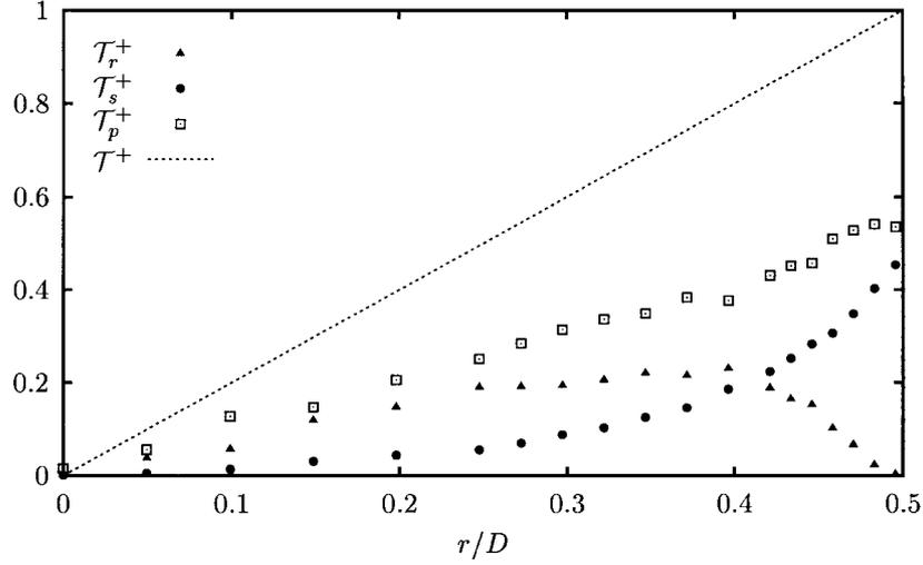
Figure 12. The various contributions to the shear stress as a function of the pipe radius for the 175 wppm solution.  $\mathcal{T}_r^+$ : Reynolds stress;  $\mathcal{T}_s^+$ : solvent stress;  $\mathcal{T}_p^+$ : polymer stress;  $\mathcal{T}^+$ : (theoretical) mean shear stress.  $Re_w \approx 9800$ .
