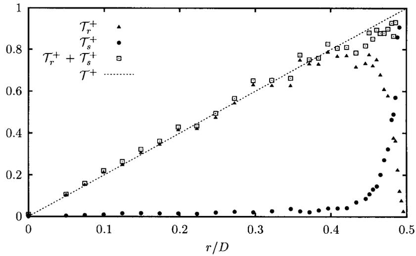
Figure 9. The various contributions to the mean shear stress for water as a function of the pipe radius.  $\mathcal{T}_r^+$ : Reynolds stress;  $\mathcal{T}_s^+$ : solvent stress;  $\mathcal{T}^+$ : (theoretical) mean shear stress.  $Re \approx 9600$ .
