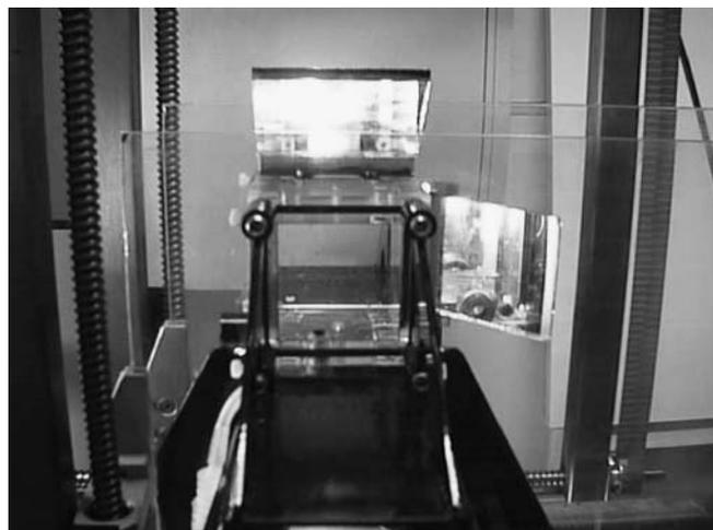
Fig. 1. The three-dimensional mixing cavity made of PMMA; clearly visible are the side and top mirrors
