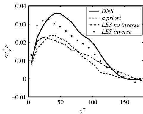
FIG. 2. Time-averaged wall-normal particle velocity as a function of the distance to the wall in wall units for  $\tau_p^+ = 5.4$ .
