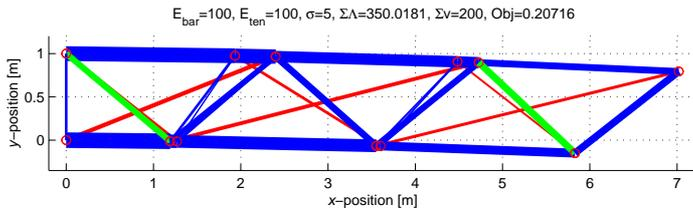
Figure 2: Optimal topology/geometry, displacement under load
