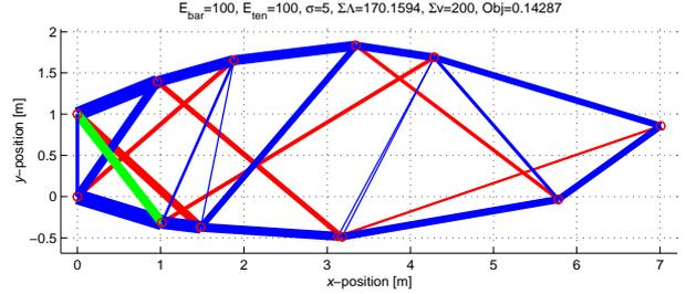
Figure 7: Optimal topology/geometry, displacement under load
