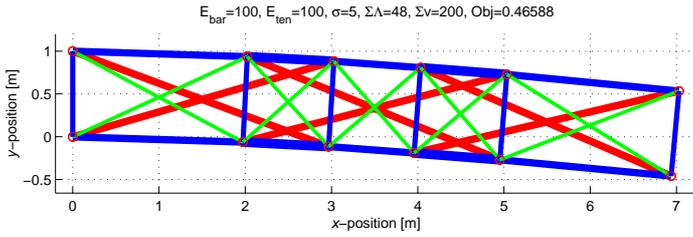
Figure 1: Basic tensegrity beam system (not optimized)
