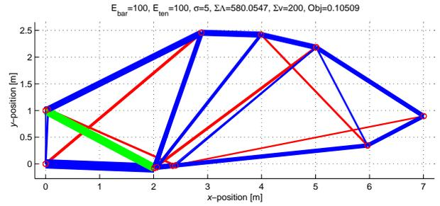
Figure 8: Optimal control/top/geo, displacement under load
