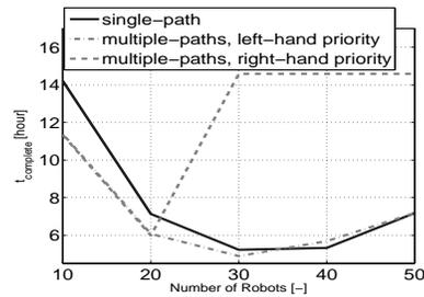
Figure 3: Comparison of  $t_{complete}$ . The priority means that at the junction robots that come from the right or left side of the other robots get higher priority
