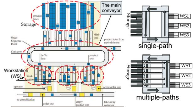
Figure 2: An Automated Distribution Center. At the right side are shown two possible geometric paths of the robots
